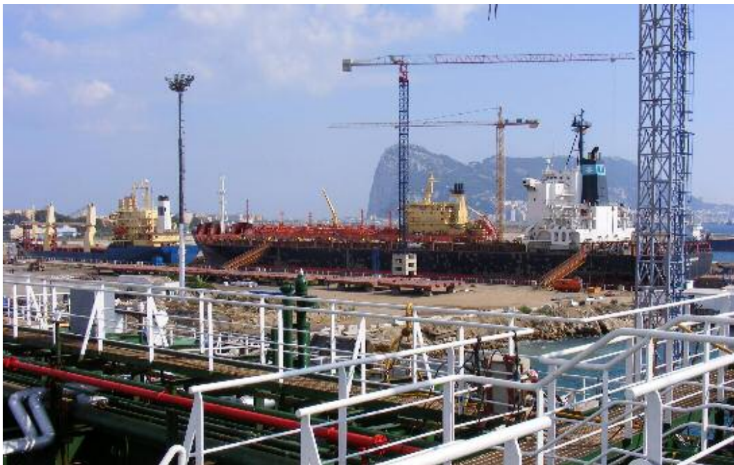
The MV " BISKRA " belonging to MARITEC N. V., Belgium, under steel and paint works, and building of rudder in CERNAVAL Shipyard, in Algeciras, Spain.
