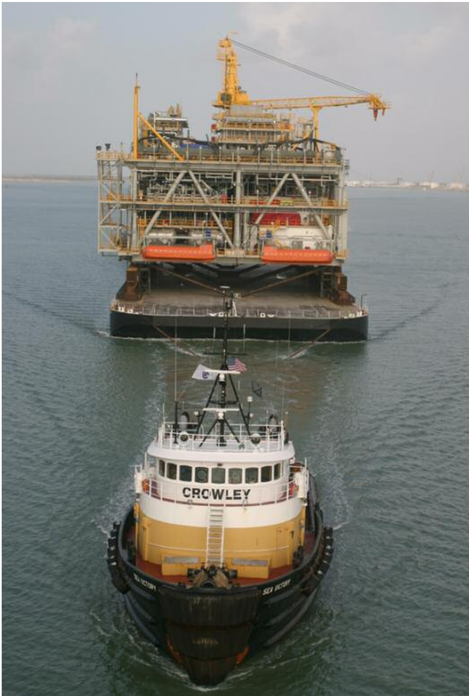
Crowley's tug Sea Victory tows one of the company's new heavy lift deck barges with an oversize production module for Chevron's Tahiti energy project in the Gulf of Mexico.
