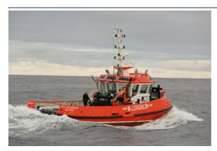
Macduff Shipyards, Scotland, have completed construction and trials on their latest newbuilding, and will deliver the recently named 'Sally McLoughlin' to John McLoughlin and Son. The 16-metre general-purpose harbour tug has a gross tonnage of just 46 tonnes with a bollard pull of 23 tonnes. The vessel is powered by twin Doosan 4V222TIH engines, through two Twin Disc MGX5222DC gearboxes to 1700mm Kort propellers. The owners are reportedly very
