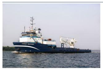
Harvey Bisso, USA, has launched operations to provide subsea services to the energy and maritime industries. The new subsea venture is a combination of Bisso Marine and Harvey Gulf International Marine. The centrepiece of the venture is a new twelve-man saturation diving system with a working depth of 300 metres. The portable SAT system will be deployed from the 81-metre by 17-metre 'Harvey Discovery', a DP2 certified multi-purpose support vessel
